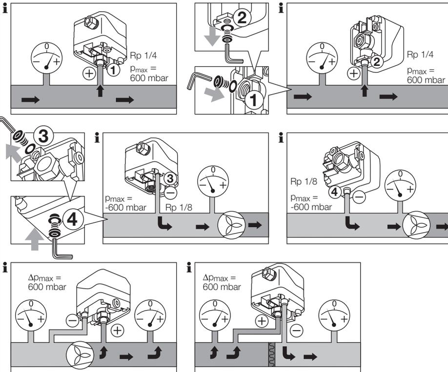
**Dichtheit prüfen****Sızdırmazlık Kontrolü****Kontrola těsnění****Kontrola szczelności****Контроль герметичности****A tömörség ellenőrzése**
